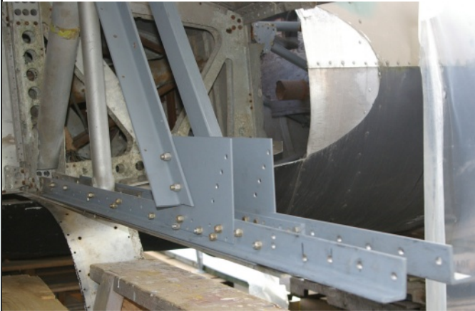
The reconstructed Hampden wing spar and fittings. Note the original metal of the engine nacelle in the background, showing the corrosive effects of 30 years on the sea bed.
