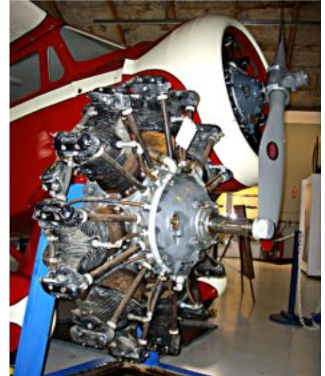
A Jacobs L4 engine, retrieved from storage and cleaned up for TechTalk II, with the Waco Cabin in the background.
